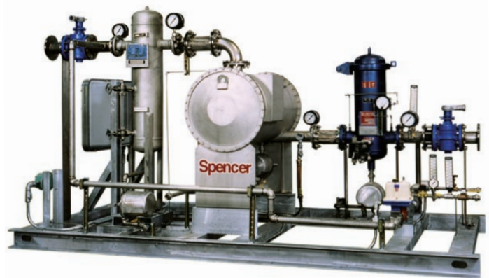
Spencer booster system installed at a California WWT plant includes a filter separator, heat exchanger and moisture separator for delivery of digester gas from maximum design volume down to "0" scfm.
