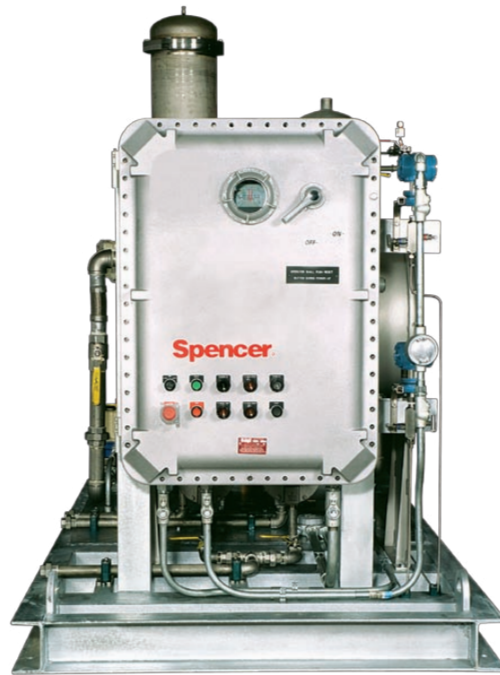
Control Panel featuring NEMA 7 enclosure controls the supply of bio-gas used as boiler fuel at a West Coast facility. It includes alarm and fault protection for high temperature and both low and high gas pressure.
