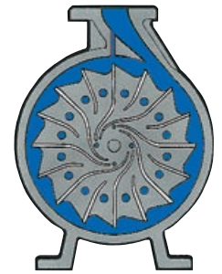
Circular concentric casing
