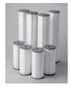
Premium quality cartridges made of pleated polyester filter media for long life and high dirt holding capacity. Cartridges can be cleaned and reused in most applications and micron ratings. Available for both 10" and 20" Big-Blue® housings. Individually shrink wrapped.
