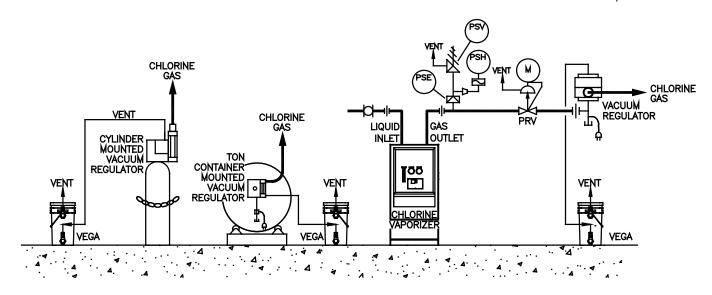
tainer with an intermediate chlorine indicator strip. When this strip turns yellow it is time to replace the first container. The second container guards against area contamination until the exhausted VEGA system can be replaced. Tests have shown that under sporadic venting conditions a VEGA system should last at least one year before replacement is required.
