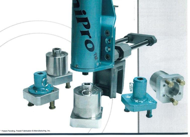
The UniPro™ Valve Closure System is pneumatic and operates even if AC power and air pressure are lost. With appropriate components in place, the system can be configured to close valves within 10 seconds in the event of a gas leak, car movement, security breach, fire alarm, seismic event or numerous other circumstances, effectively stopping the leak well before escaping gas becomes a hazard to those on-site or in the surrounding community.
